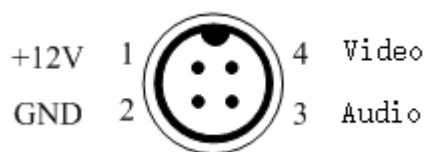
AV-OUT Monitor Interface
