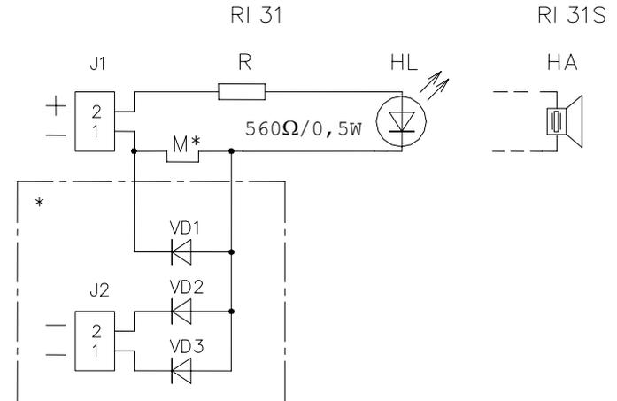
\* Three input control option; the bridge M has been cut off.
